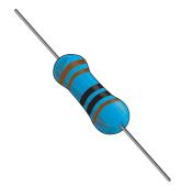
If the three bands are brown, red and blue this would translated to 126. The forth band is the multiplier. You multiple the first three digit by this band and then you get the resistance of your resistor. The fourth band follows the below color scheme:
