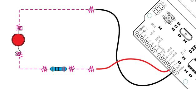
This is commonly how you color code your cables while working with electronics. Red is used to mark a cable that connects to the power out and black are used to mark cables as ground cables. All of the following examples used in this book will follow the same color scheme. Note that red cables does not mean that they are always connected to the digital pins. In this example we are switching 5V on and of on the digital pins and that is why we used red to mark the cable.
