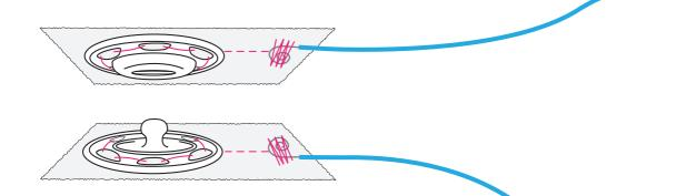
The last hidden button is made like a normal button. The trick is to yet again to use conductive thread to sew the button in place and then sew around the button hole using the same thread. Most modern sewing machines have a preprogrammed function for making button holes and will work perfectly for this. Just load you machine with conductive thread and cut the hole in the fabric. This example works the same way either with a normal sew-on button or a jeans button.
