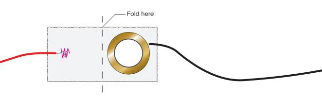
Now we have a piezo speaker that is a bit softer than a normal one and we can get started on some programs to generate sounds. To make the vibrations that generates sound we will pulse the piezo with power. To make these pulses fast enough to generate vibrations we cant use the normal delay() since this pause isn't quick enough. Instead we will use delayMicroseconds(). In the following example we will generate a vibration that creates the tone A:
