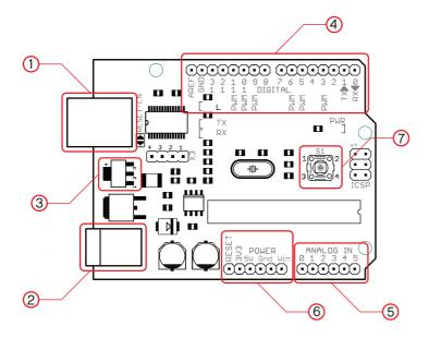
The USB connector (1) is used for connecting your Arduino board to your computer. While connected the Arduino board will be powered from the USB cable and while connected you can upload code and you can communicate from and to your Arduino board.
