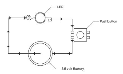
The power from the battery will travel through the cable into the LED in one leg and out the other down to the button and back to the battery.
